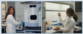
**GC-MS (Gas Chromatography - Mass Spectrophotometer)** The GC-MS machine is primarily used to test for pesticides and PCBs. It is also used for the identification and quantification of oils, and for volatile samples including EPA and DHA.
