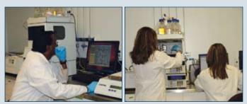
ICP (Inductively Coupled Plasma) The ICP machine is used to measure minerals and heavy metals.
